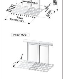
(These detection patterns are approximate and will vary slightly. Walk-test the unit to assure the pattern desired.)
