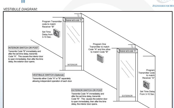
can not only be used to activate automatic doors, but can also be used to directly release electric locking devices or sequence electric locking devices on automatic doors without any additional relays or timers.
