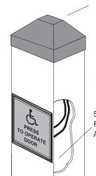
DIRECTLY UNDER PLASTIC END CAP FOR OPTIMUM PERFORMANCE AND EASE OF BATTERY REPLACEMENT
